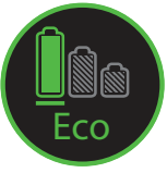
The screen showing the machine set to Eco mode with a full battery in green to show that this will give the longest battery life of the three modes.
